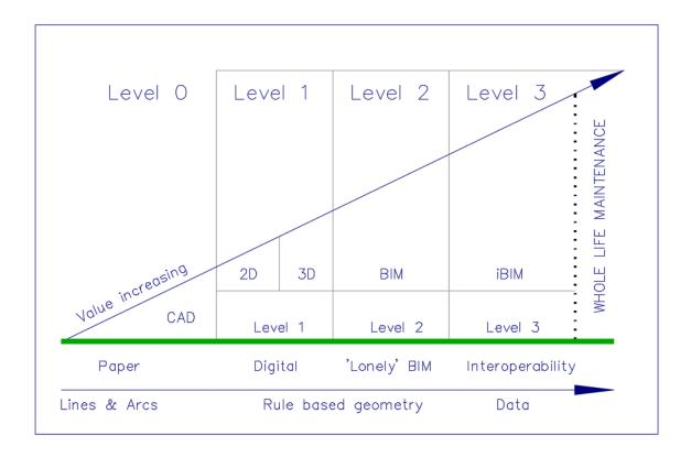
As we move the design process from one done on paper, to 2D CAD and so on, the opportunities for the model to add business values become clear. Ramping up the level at which we work, we move through 'lonely' BIM, with little or no interoperability, through to integrated BIM (iBIM), with a high level of interoperability, integration and business value. Few, if any schemes have been operating at Level 3.
