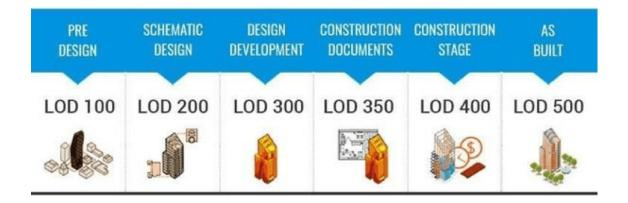
The American Institute of Architects has a framework that uses numbers (see above). Whichever framework is employed, it is clear that these stages are useful as descriptions of design elements during a single Design, Build and Commission iteration. The as-built model can then add enormous value at the start of any future iteration, so it is incredibly important to get this right before it is passed on to the owner/operator.
