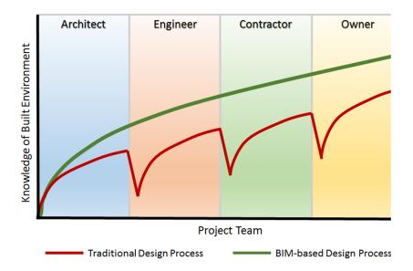
The ideal is to make sure no information is lost at any stage, saving time and reducing error. The information should also become richer as time progresses. This increases the level of understanding between interested parties. In the design and construct phases good data management can reduce the frequency and cost of expensive last minute design changes.
